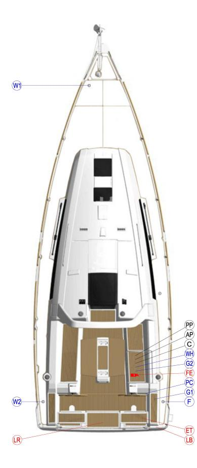
Construction year: 2014 Length: 11.5 m Beam: 4.0 m Draft: 2.1 m Fuel capacity: 130 l Water capacity: 336 I - Tank 1: 206 I - Tank 2: 130 I
